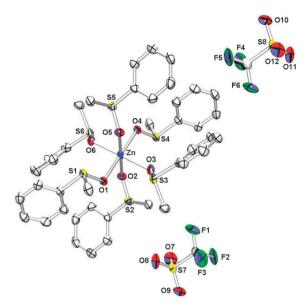
Fig. 1 Molecular structure of  $Zn(5)_6(OTf)_2$  (29). Hydrogen atoms are omitted for clarity. Thermal ellipsoids are drawn at the 50% probability level. Selected distances (Å): Zn-O(1,2,3,4,5,6): 2.0817(14), O-S: 1.4265(18).
