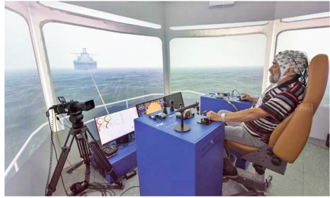
Fig. 2. Simulator Setting with 360° projections
