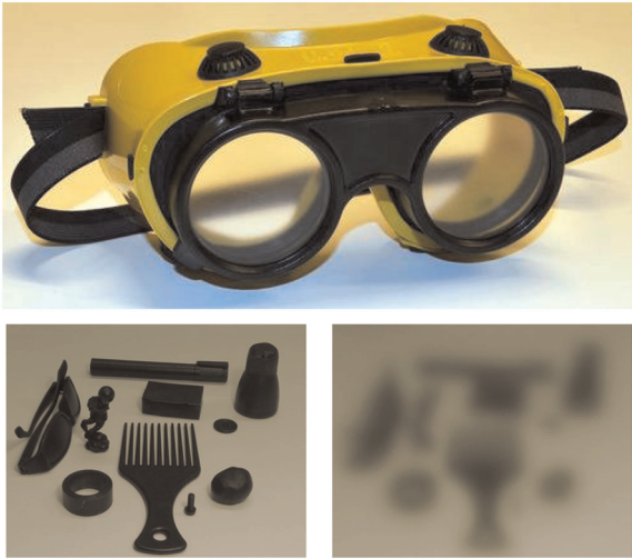
Fig 2. A goggle with blurring glasses was used to impair vision. The images below show the resulting view of the target objects by the participants in the control condition (left) and the impaired condition (right).
