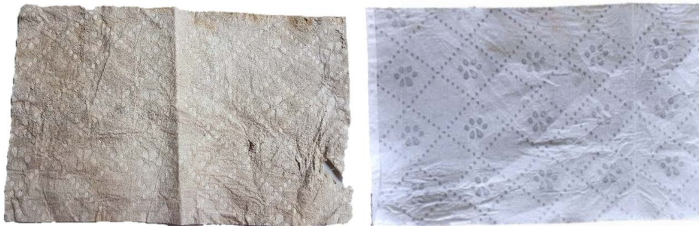
Figure 4-26: Left side: Staple fibre nonwoven found in pump blockage. Right side: Reference sample of moist toilet wipe sold as flushable
