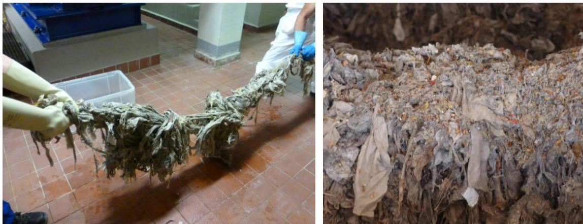
Figure 1-1: Blockage removed from a Berlin pumping station (left) and screenings from a Berlin WWTP (right)
