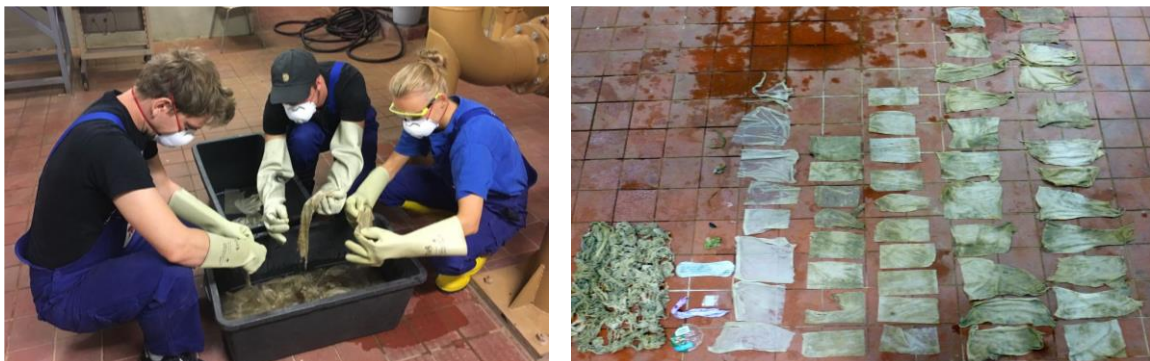
Figure 3-4: Left: Disinfecting, rinsing and sorting of blockage material; right: Constituents of pump blockage, sorted into fractions
