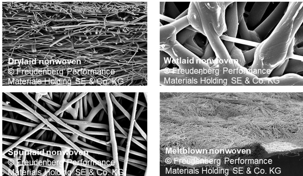
Figure 2-1: Photomicrographs of different types of nonwoven fabrics by web formation type [16]
