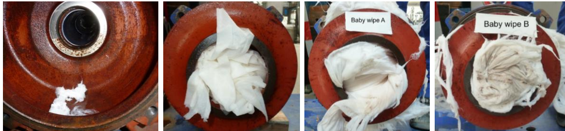
Figure 4-37: Laboratory test pump clogged with different nonwoven wipes From left to right: Toilet wipe B, Toilet wipe C, Baby wipe A, Baby wipe B
