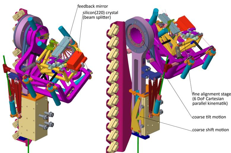
**Prototype testing** - The Investigation of the prototype showed, that the positioning mechanics as well as the laser interferometer measuring system in general works. In order to obtain quantitative results, the test set-up will be transferred into a vacuum environment. Using a thermal camera, the induction of heat due to the friction between the lead screw and the nut for the vertical shift could be visualised (maximal gradient < 1 K).
