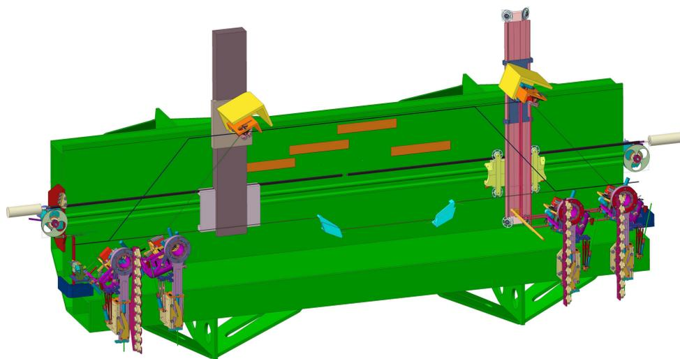
**Optical bench** - The optical bench suits as support structure, carrying the mechanics for positioning the optical elements and other components such as monitoring and measuring systems. It is designed with maximal stiffness and with as much separation from the chamber as possible - thus providing a most stiff and stable support structure with minimised disturbing influences.
