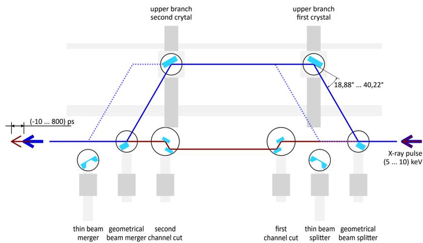
**General concept** - Showing a conceptual view of the SDL's beam path and indicates the mechanical concept.
