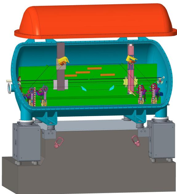
**General design of the SDL at its current state** - Showing the optical bench with the crucial optomechanics, installed inside a cylindrical vacuum chamber with the dimensions of about (2 x Ø1) m. The chamber stands on a granite block for a most stable grounding. Half of the cylindrical shell can get tilted up, providing a wide and comfortable access to the mechanics.
