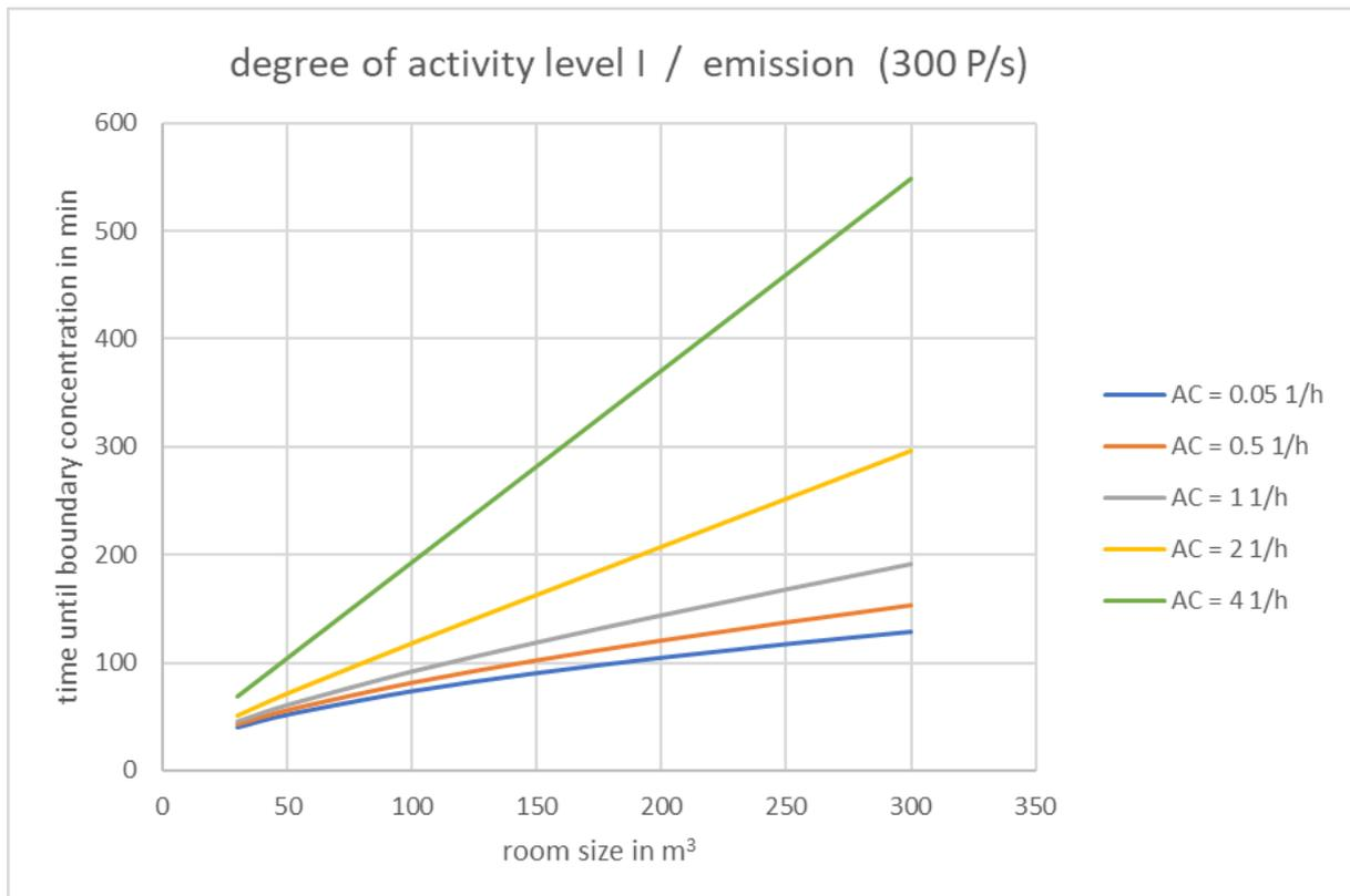
Figure 2: time in minutes until the number of inhaled virus exceeds 3,000 virus depending on the room volume and the air change
