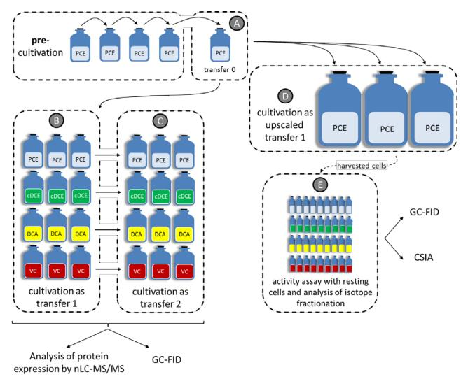
**Figure S1: Experimental setup exemplified for pre-cultivation with PCE.** Identical procedures were done for pre-cultivation with cDCE, DCA and VC.
