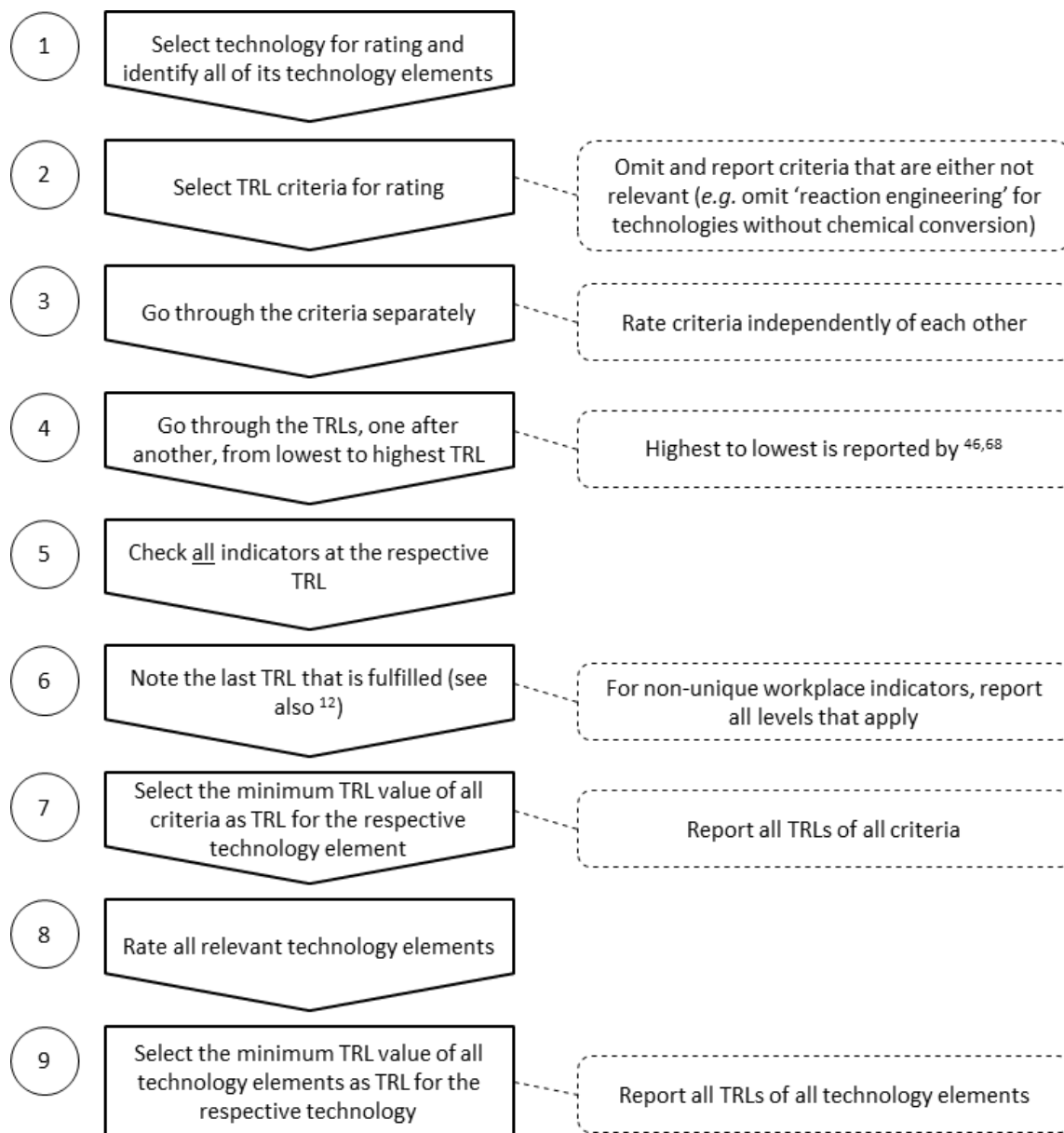
Figure 4: Stepwise approach for TRL rating of technology elements (steps 1-7) and composed technologies (steps 8-9)
