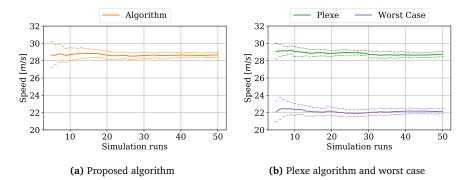
**Figure 4.6** – The average speed depending on the number of simulation runs (solid line) and the corresponding 0.95 confidence intervals (short horizontal lines) for (a) the proposed algorithm and (b) the Plexe algorithm and the worst case.
