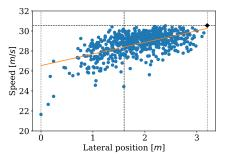
**Figure 4.9** – Correlation between the platoon's lateral position and its average speed for 650 simulation runs. The line is a linear function and the black diamond in the upper right corner indicates the platoon's limits due to its desired speed of 30.6 m/s and the center of lane two at 3.2 m.
