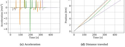
**Figure 4.4** – Detailed results of a single simulation run with medium traffic and a platoon of length four: the platoon's (a) speed, (b) lane position (dashed black lines indicate lane markings), (c) acceleration, and (d) distance traveled.
