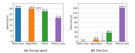
**Figure 4.3** – The results of a (non-representative) single simulation run with medium traffic and a platoon of length four: the platoon's (a) average speed and (b) time loss.
