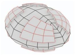
FIG. 7. A discrete ellipsoid  $(n_1, n_2 \text{ integer}, n_3 = \text{const})$  from the system (53) and its two adjacent layers from the dual n  $(n_1, n_2 \text{ half-integer}, n_3 = \text{const} \pm \frac{1}{2})$ . All faces are planar and orthogonal to the corresponding edges of the other net.
