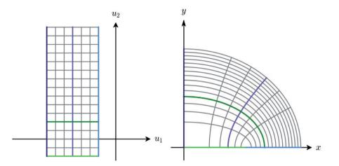
FIG. 3. Square grid on the domain  $\mathcal{U}$  and its image under the map (47). The horizontal lines  $u_2 = const$  are mapped to ellipses with the degenerate case  $u_2 \searrow -b$ , which is mapped to a line segment on the *x*-axis. The vertical lines  $u_1 = const$  are mapped to hyperbolas with the degenerate cases  $u_1 \nearrow -b$ , which is mapped to a ray on the *x*-axis, and  $u_2 \searrow -a$ , which is mapped to the positive *y*-axis.
