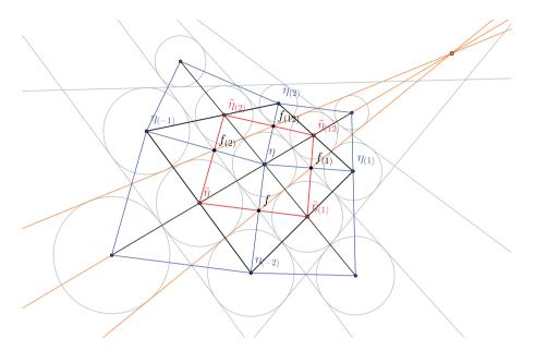
FIG. 9. Koenigs property of the incentre net  $\omega$  of an IC-net implies the Koenigs property for its two diagonal nets  $\eta$  and  $\tilde{\eta}$ .
