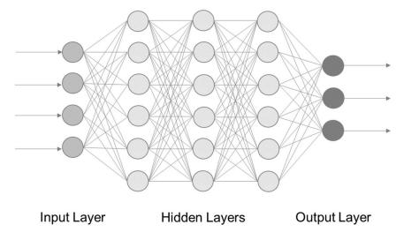
**Figure 3.** Architecture of a feedforward neural network with four input neurons, and three output neurons, and (here exemplarily three) hidden layers [40].
