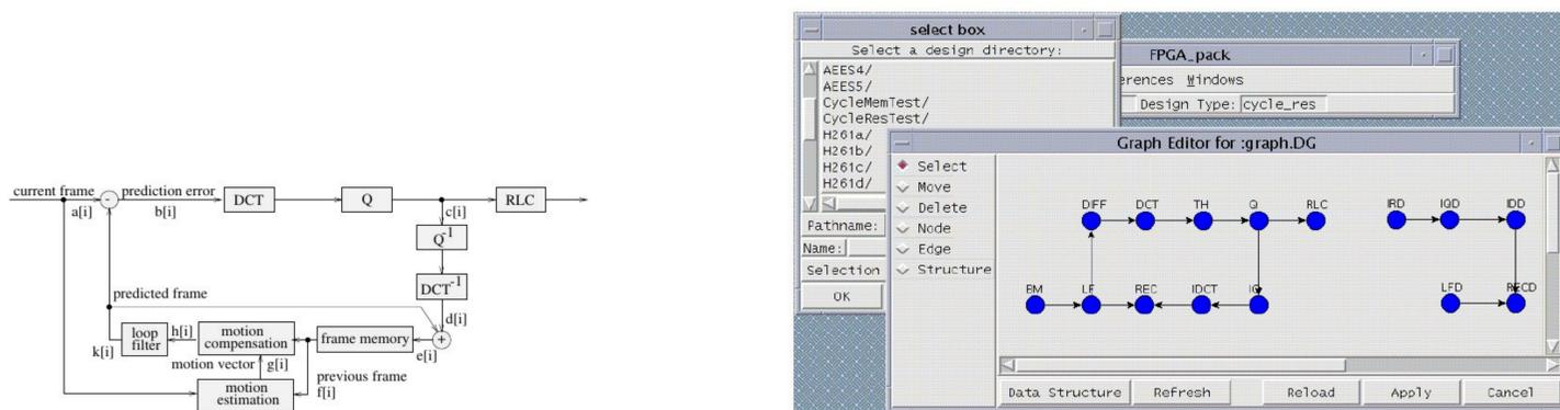
Figure 7: Block diagram of a video-codec (H.261) (left); problem graph of the video-codec (right).
