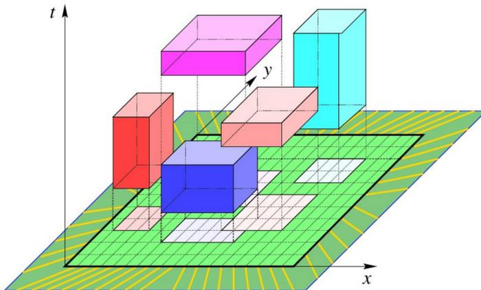
Figure 1: An FPGA and a set of five jobs, shown in ordinary two-dimensional space and in three-dimensional space-time. Jobs must be placed inside the chip and must not overlap if executed simultaneously on the chip.
