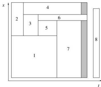
Figure 2: A set of jobs that is feasible for scheduling with one resource constraint, but infeasible for two-dimensional packing: Job 8 does not violate a resource constraint, but does not fit as a contiguous rectangle.
