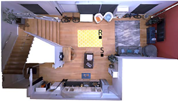
Fig. 6. Top view of the room used for the measurements in the PIV and TDOA comparison. The visualization is part of the Replica Dataset [29] and the furniture was in a different configuration during the acoustic measurements. Approximate source (S) and receiver (R) locations are marked as black squares.
