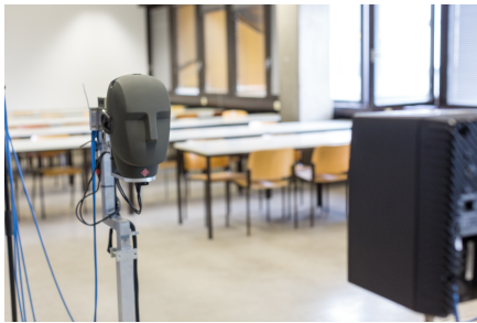
Fig. 2: Measurement of the HRTF set in the seminar room at TH Köln using a Neumann KU100 artificial head mounted on the VariSpear device.
