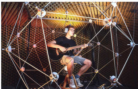
Fig. 2: Surrounding spherical microphone array used to capture the direction-dependent sound.
