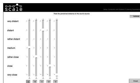
Fig. 7: User interface of the experiment. The left side displays the seven-point category scale. The five faders correspond to the five actual measured distances, randomly ordered for each trial.
