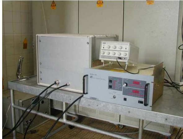
Figure 3.4: 24 kV, 8000 J/s pulse modulator (left), power supply (right) and frequency generator (top of power supply)
