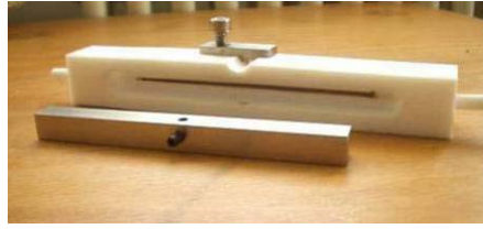
Figure 3.6: Parallel plate continuous treatment chamber with stainless steel electrodes and Teflon insulator, 2 mm electrode gap.
