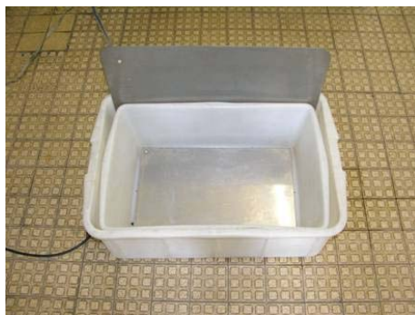
Figure 3.8: Batch PEF-treatment chamber with a volume of 25 l
