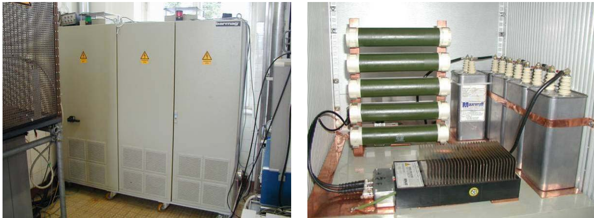
Figure 3.3: 20 kV, 40 kJ/s power supply (left) and pulse modulator internal view (right), showing thyristor switch in the front, five parallel protective resistors and a setup of capacitors in series.
