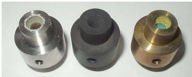
Figure 4.71: Electrodes of colinear treatment chamber with an inner diameter of 6 mm after 21 days continuous operation time at 20 kV/cm, 100 kJ/kg and a flow rate of 5 kg/h. Stainless steel, graphite and copper-beryllium (left to right).
