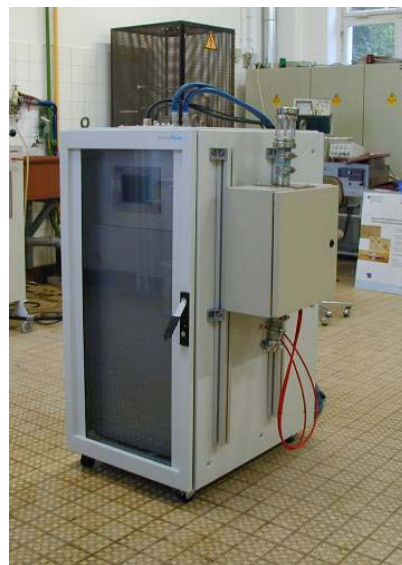
Figure 3.5: Rectangular pulsed power modulator, 50 kV peak voltage, 200 A peak current, 400 Hz.
