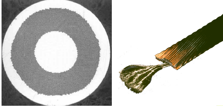
Figure 2.3: LHC Main Bending Magnet (MB) strand and cable. (left) strand cross-section featuring a copper core, Nb-Ti filaments (dark spots) embedded in the copper matrix and a copper coat. (right) Rutherford-type cable. The filaments of one strand are separated from the copper matrix by etching. Courtesy of CERN ©.
