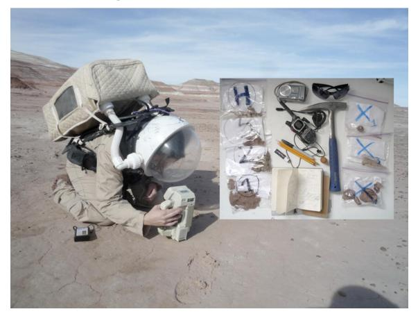
Figure 5.23: Problems with geological instrument interaction at MDRS, 2010: The instrument monitor is not visible because of solar light and helmet; the interface is not usable with EVA gloves; the instrument's design should be dedicated to the particular human-machine-environment interaction of space. It is not convenient to adapt earth instruments for use in space exploration.
