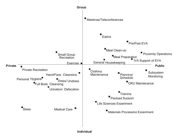
Figure 2.15: Locations of space module functions with functional relationships analysis (AA.VV., 1999b, SSP50008, MSIS-86, Figure 8.3.2.2-2). Grouping the activities according to psychological and physiological needs (private, public, group, individual) is fundamental for increasing habitability.
