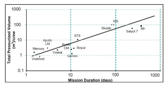
Figure 0.5: Spacecraft pressurized volume (NASA, 2010b p. 562, Figure 8.2-2)
