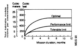
Figure 0.4: Guideline for Determination of Total Habitable Volume per Person in the Space Module (NASA-STD-3000 90 from AA.VV., 1999b, SSP 50008, Figure 8.6.2.1-1)
