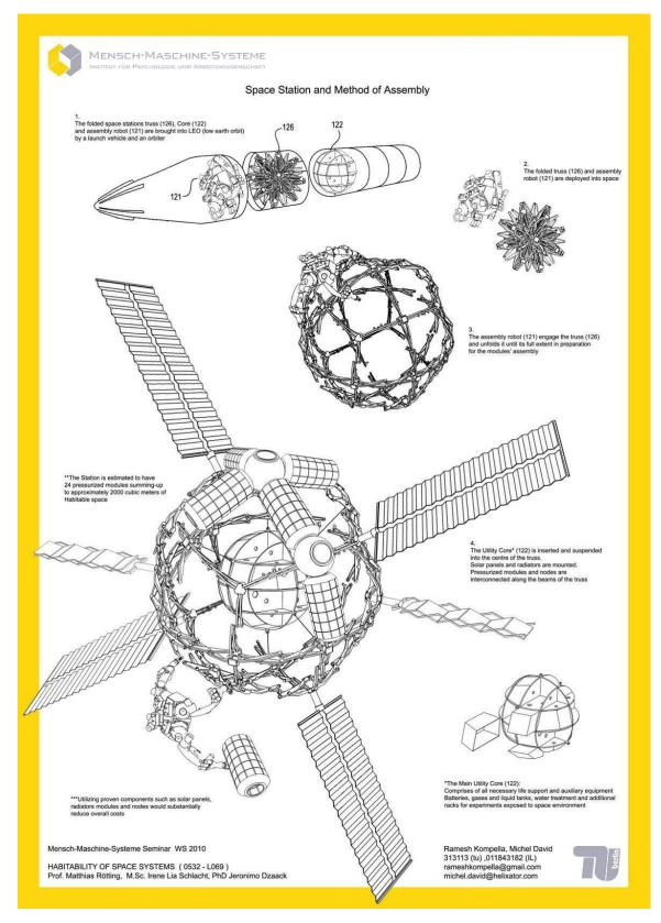
Figure 5.26: Space station and assembly method. Michel David, Ramesh Kompella under the tutoring of I.S. Schlacht MMS Seminar WS 2010 TU-Berlin.
