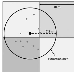
**Figure 4.** Exemplary extraction area of 176.7 m<sup>2</sup> with 10 m pixels in the background. The center of the circle represents the centroid of the sampling locations of all dates (grey dots).
