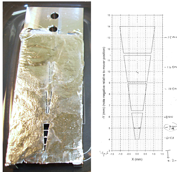
Figure 2.9: Left: picture of the LCLS slotted spoiler foil. The lowermost slot is the single slot. It is V-shaped to adjust the pulse length of a single pulse. The slots above it are double slots to produce two x-ray pulses separated in time. Right: drawing of the single slot
