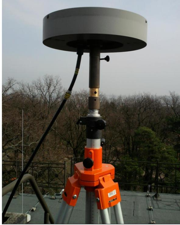
Figure 3.3: Equipment for the vertical movement experiment of a GNSS antenna
