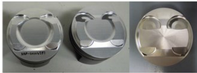
Figure 2.2: Examples of the pistons used during testing to vary compression ratio. From left to right 10.2:1, 11.2:1 and 12.2:1
