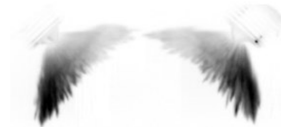
Figure 2: View of the fuel atomization with the use of two angularly arranged injectors
