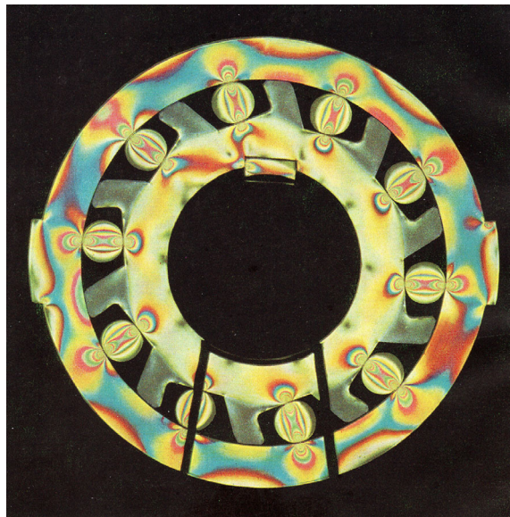
FIGURE 3 Isochromats in a freewheel model obtained in the photoelasticity laboratory of Ludwig Föppl. A torque acts clockwise on the outer ring. This causes the rollers to jam between the sloped surfaces of the inner ring and the outer ring. Model made of unsaturated polyester resin VP 1527, 10 mm thick, diameter 230 mm. Reproduced from [7]
