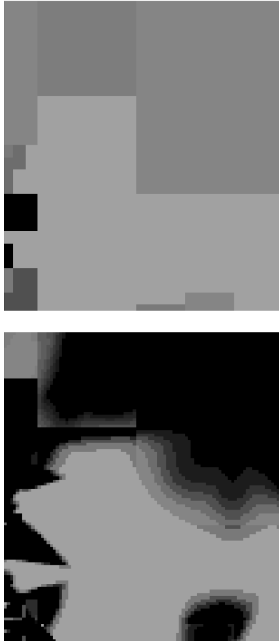
Figure 5.27: Top : Block-based motion vector field for reference list 0 of the upper left part of frame 7 of the BQSquare sequence. Bottom : Interpolated motion vector field of frame 7. A grayscale version of the x-component of each motion vector is shown.
