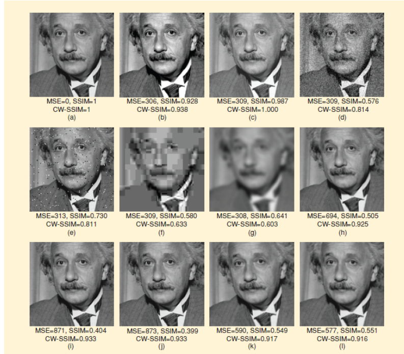
Figure 2.3: "Comparison of image fidelity measures for "Einstein" image altered with different types of distortions. (a) Reference image. (b) Mean contrast stretch. (c) Luminance shift. (d) Gaussian noise contamination. (e) Impulsive noise contamination. (f) JPEG compression. (g) Blurring. (h) Spatial scaling (zooming out). (i) Spatial shift (to the right). (j) Spatial shift (to the left). (k) Rotation (counter-clockwise). (l) Rotation (clockwise)." Source: [51].
