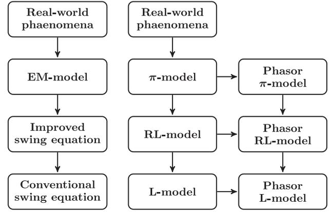
FIG. 1. Model hierarchies for synchronous generators (on the left) and transmission lines (on the right).
