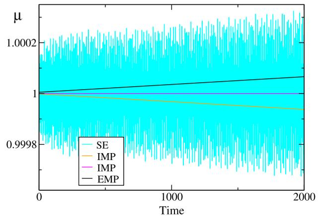
FIG. 2. Conservation of Lagrange multiplier  $\mu$  for different integration schemes [Symplectic Euler (SE), Implicit Midpoint (IMP), Explicit Midpoint (EMP)] and  $K = 0.5$ . The orange and magenta curves differ in the convergence threshold in the nonlinear solver ( $10^{-6}$  and  $10^{-12}$ ).
