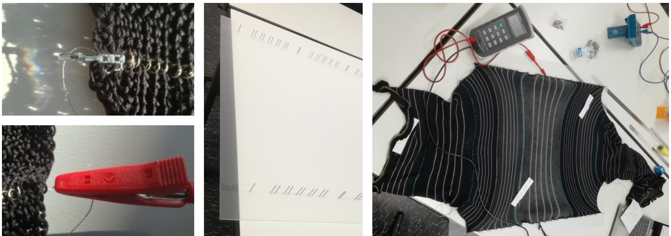
Figure 3. Resistance measurement: unsatisfactory crimp connection ( left, top ), alternative method using clamps ( left, bottom ), fastening device ( middle ), fastening device with mounted test vehicle and multi-meter measuring setup ( right ).
