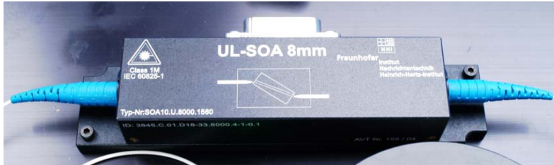
Figure B.1.: Packaged 8 mm-long UL-SOA module (left) fabricated and assembled at the Heinrich-Hertz-Institut; the 8 mm-long UL-SOA chip is mounted on a heat sink (right) and is connected electrically from the top with wire bonds and optically from the left and right due to fibre coupling
