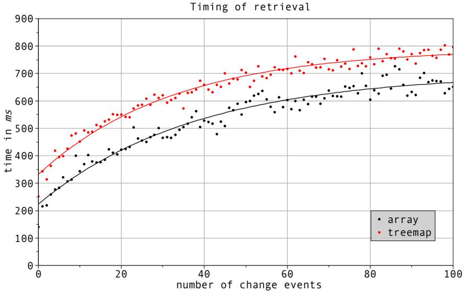
Figure 1: Comparison of the runtime performance for two different implementations of the network change event retrieval. The array based approach using binary search is about 20% faster than the approach using a Java TreeMap. The complexity of both approaches is  $O(\log n)$ .
