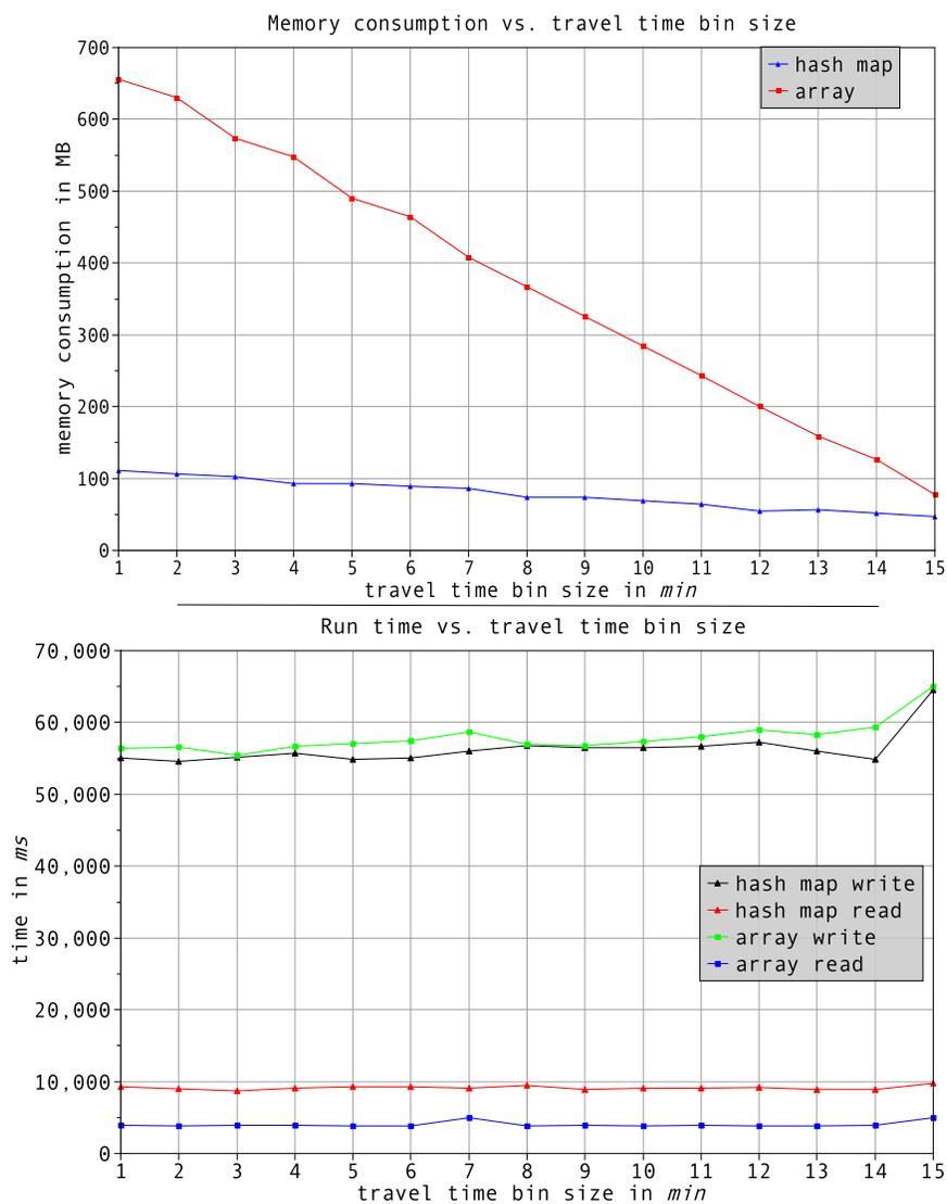
Figure 2: Comparison of two different implementations of the storage and retrieval mechanism for the time dependent link travel times. Top: comparison of the memory consumption. The Java HashMap based approach consumes considerable less memory than an array based implementation. Bottom: comparison of the runtime performance. For write operations both approaches have almost equal execution times. The array based approach is faster for read operations.
