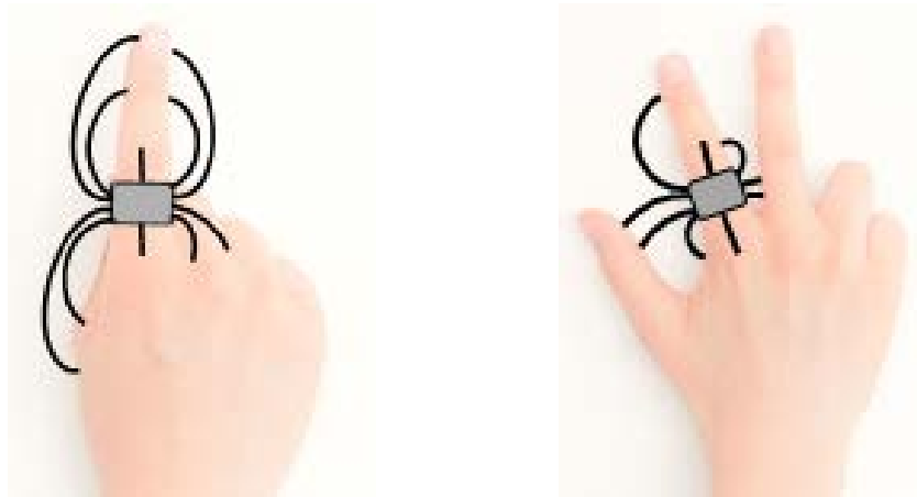
Figure 5.1.: Visualization of the basic idea: The ring creates electric fields around the ring. Depending on the finger pose, the fields are different influenced.
