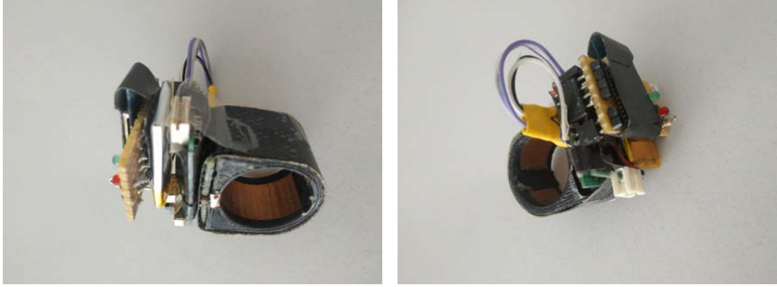
Figure A.11.: First self-sufficient PeriSense prototype with TI FDC1004, Invensense MPU9250, Bluetooth module, and Battery.
