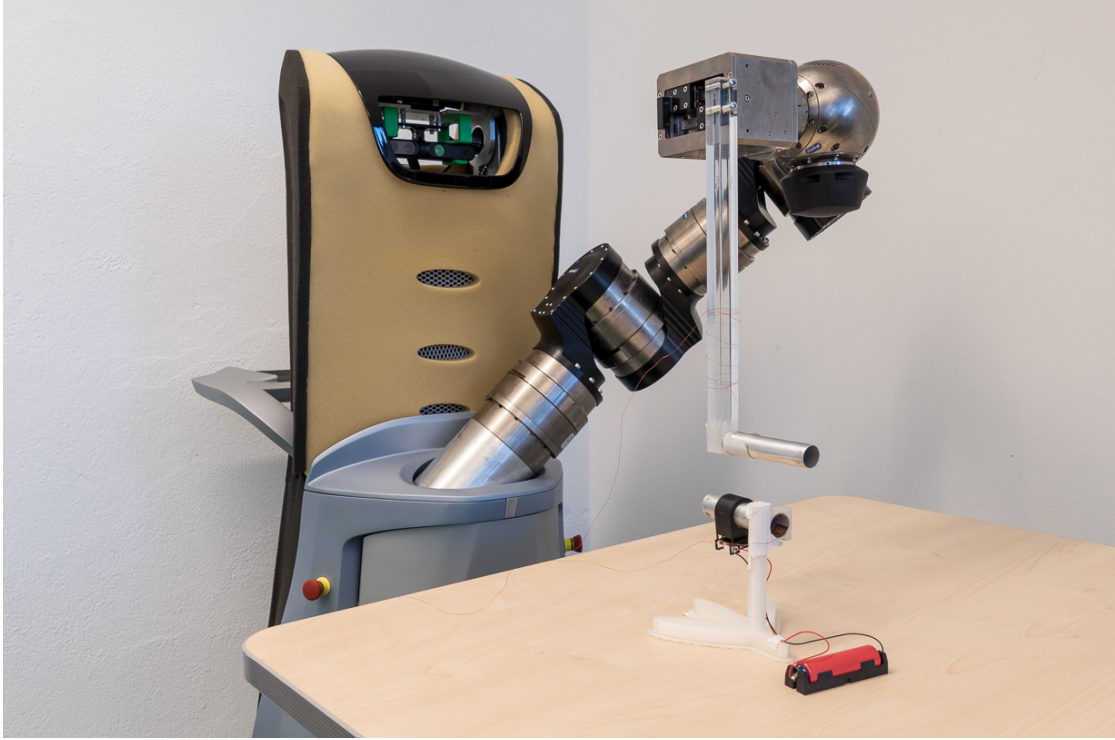
Figure 6.4.: Experimental set-up for evaluation of spatial sensor resolution.
