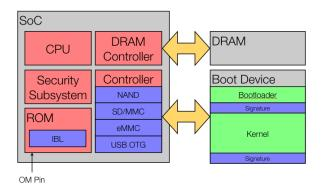
Figure 2: Boot architecture on mobile devices. The OM pin determines the boot medium. The IBL initializes the DRAM and the boot medium controller and loads the bootloader into the RAM. The security subsystem may be used to speed up signature checks.
