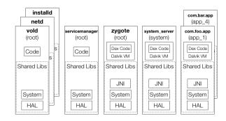
Figure 4: Schematic figure of the processes running in an Android system. Some services run with root privileges which makes them a valuable target for root exploits.
