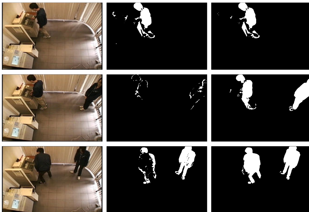
Figure 5.9: Foreground segmentation results for three frames of the 'copyMachine' sequence. From top to bottom: frames number 147, 824 and 2686. From left to right: original frame, foreground mask of SGMM and foreground mask of SGMM-SOD.
