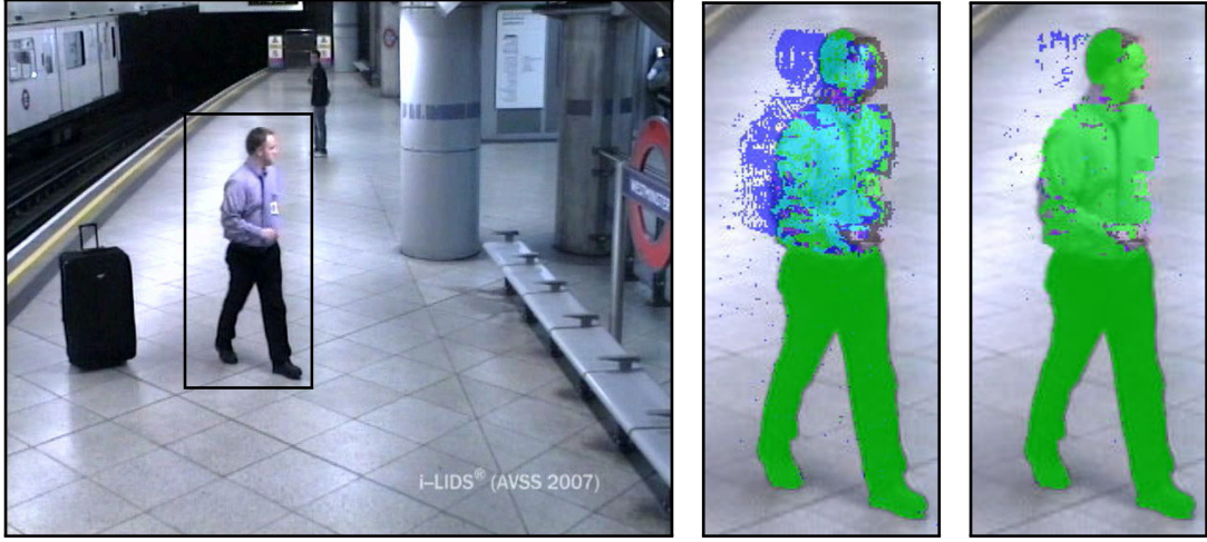
Figure 4.4: Multi-class pixel classification. From left to right: Frame number 2637 of the i-LIDS (AVSS 2007) AB-Easy sequence, detail of pixel classification using the FSM depicted in Figure 4.2, and using specialized states (Figure 4.3). Pixels are colored attending to their classification.
