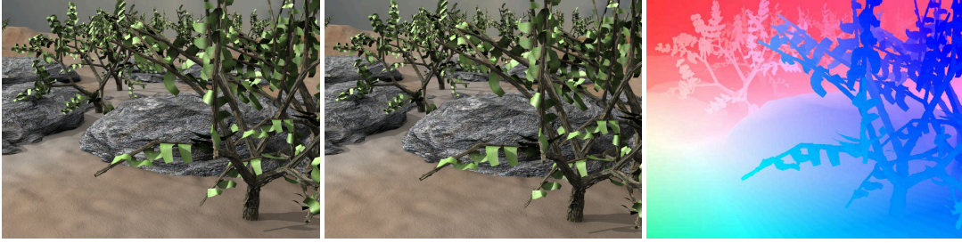
Figure 1.4: Optical flow example for two frames of the sequence 'Grove3' from the Middlebury dataset. From left to right: frame number 9, frame number 10, ground-truth flow (source, http://vision.middlebury.edu/flow/ ).
