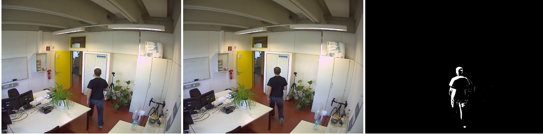
Figure 1.2: Temporal differencing. From left to right: first image of a pair containing one moving person, second image of the same image pair, and difference mask.
