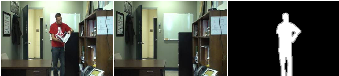
Figure 1.3: Background subtraction example for two frames of the sequence 'office' from the CDnet dataset. From left to right: frame number 001835, background of the scene, and ground-truth foreground mask (source, www.changedetection.net ).
