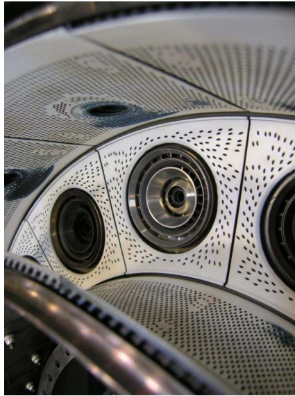
Figure 2.3: View into the annular combustor of the Rolls-Royce E3E Core 3/2 technology demonstrator, optimized for lean burn combustion and NO x reduction. (Courtesy of Rolls-Royce plc.)
