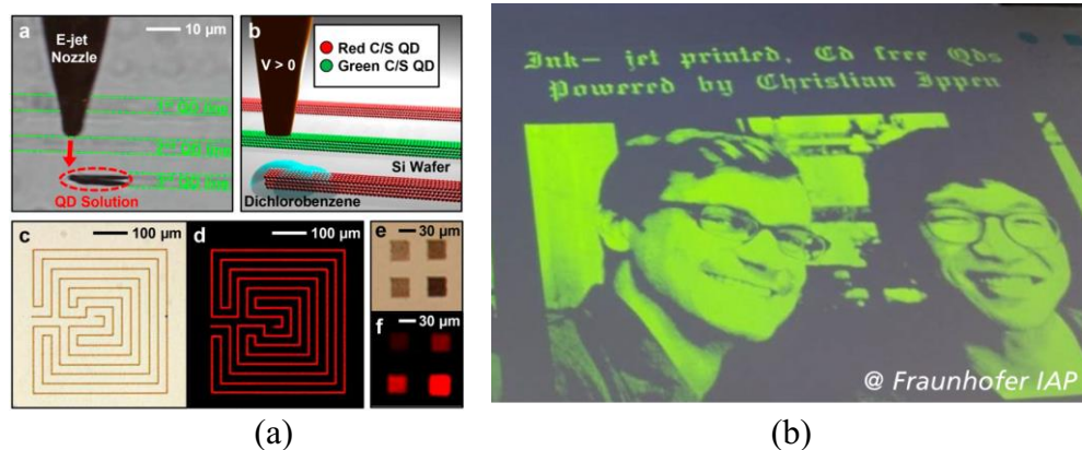
Figure 1.1.2 (a) E-jet printed homogeneous QD array with a pixel size of 30 \times 30 \mu\text{m}^2 using CdSe-based QD inks [18] and (a) an inkjet-printed picture on paper with InP-based QD inks.
