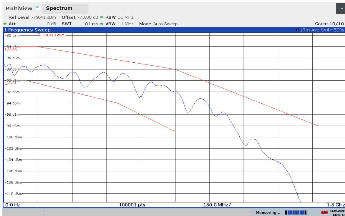
Figure 5.37: The power spectral density analysis of the PRBS data of PAM-4 running at 2.8 Gb/s and the IEEE Automotive Ethernet limit lines plotted on the graph as well.
