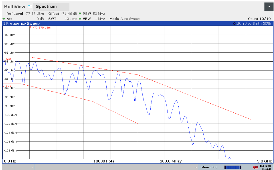
Figure 5.36: The power spectral density analysis of the PRBS data of PAM-4 running at 5.6 Gb/s and the IEEE Automotive Ethernet limit lines plotted on the graph as well.
