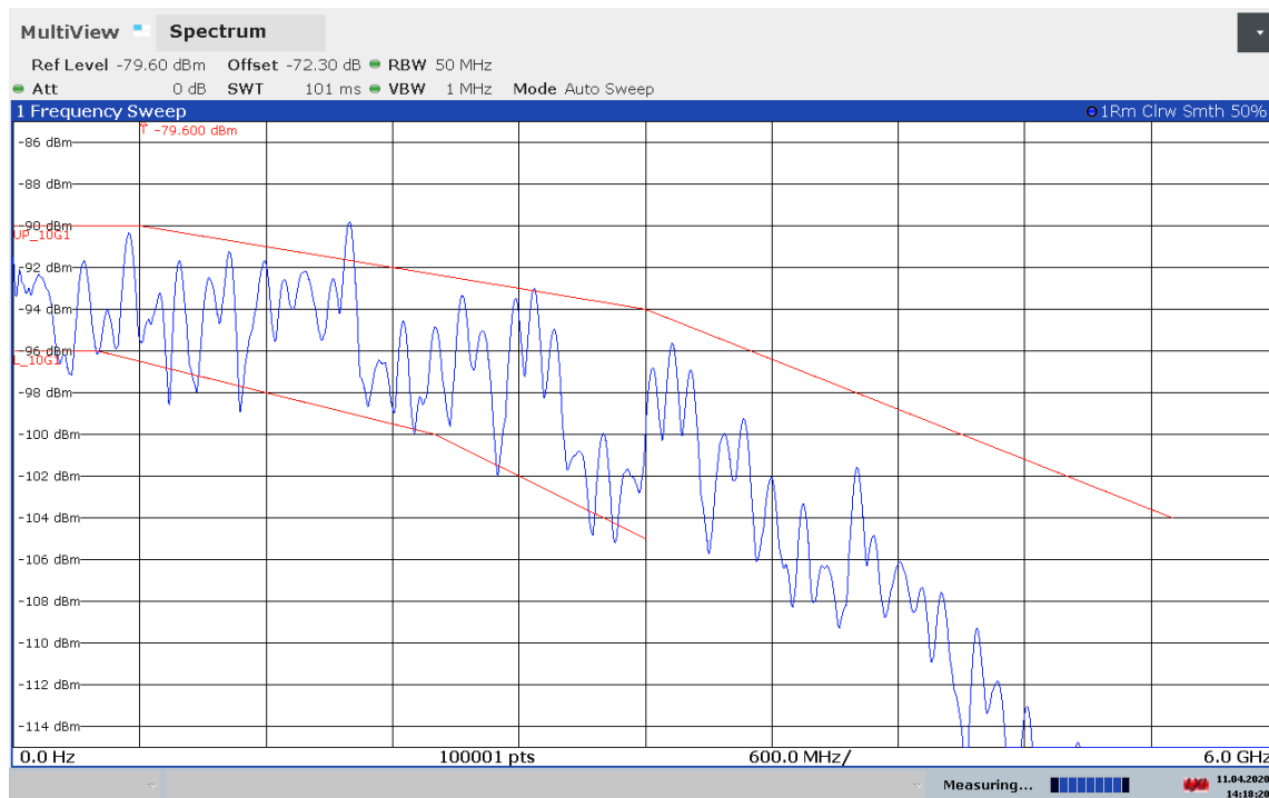
Figure 5.35: The power spectral density analysis of the PRBS data of PAM-4 running at 11.2 Gb/s and the IEEE Automotive Ethernet limit lines plotted on the graph as well.
