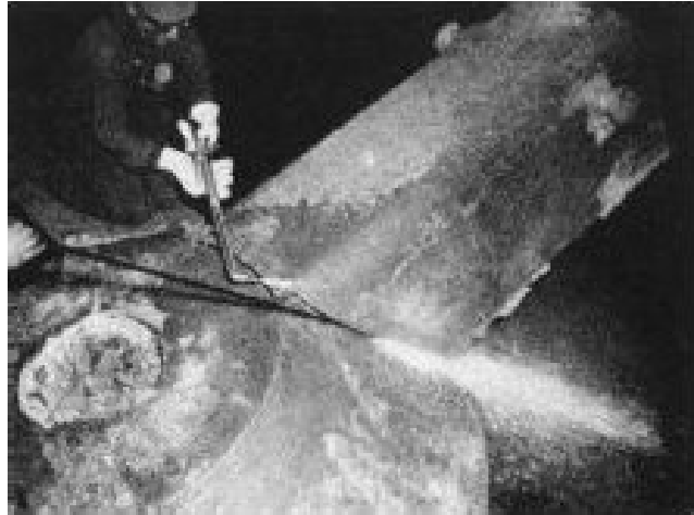
(b) Oxygen lance used in conjunction with cutting torch to remove 7 t riser from 9 t steel casting.
