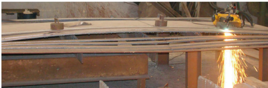
Figure 2.7: Edge buckling due to oxy-acetylene cutting [12].
