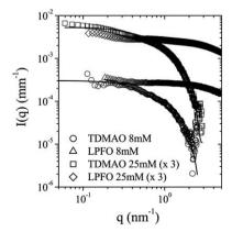
Fig. 1 Scattering from individual surfactant solutions of LPFO and TDMAO for the two concentrations reported. The scattering curves for 25 mM have been multiplied by a factor 3 for clarity.
