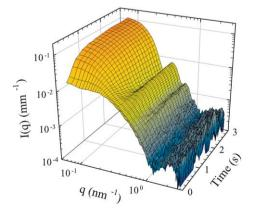
**Fig. 4** Time evolution of the background subtracted scattered intensity upon mixing 25 mM solutions of TDMAO and LPFO in a 3:4 mixing ratio (x[TDMAO] = 0.43).
