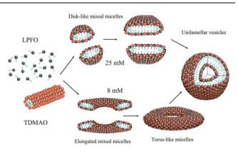
**Fig. 9** Schematic representation of the two different pathways followed in the formation of ULVs near (25 mM) and well below (8 mM) the cmc of the anionic micelles (LPFO).
