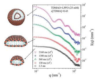
Fig. 5 Representative time-resolved SAXS intensities after mixing of 25 mM solutions of TDMAO and LPFO with x[TDMAO] = 0.43. Successive curves have been multiplied by a factor 5 for clarity. The continuous lines correspond to models described in the text. The cartoons illustrate the different aggregate shapes used to model the data.
