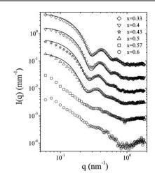
**Fig. 3** SAXS intensities of the final state at different TDMAO fractions, *x*[TDMAO], of initial 8 mM solutions of TDMAO and LPFO. Successive curves have been multiplied by a factor 3 for clarity.
