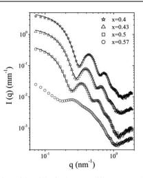
**Fig. 2** SAXS intensities of the final state at different TDMAO fractions, x[TDMAO], of initial 25 mM solutions of TDMAO and LPFO. Successive curves have been multiplied by a factor 3 for clarity.
