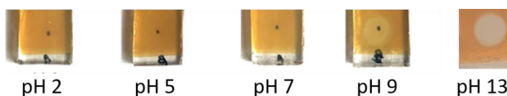
Figure C2. Photographs of \alpha -SnWO 4 films after PEC treatment in various pH electrolytes. PEC measurements were performed for 1 h with an applied potential of 1.23 V vs. RHE. Clear dissolution and exposure of the FTO substrate can be observed in alkaline conditions. A visual change cannot be observed in acidic to neutral pH. The black dot indicates the center of the exposed film area.
