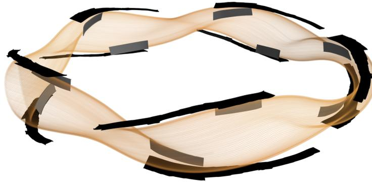
**Figure 1.2.:** The divertor plates (black) arranged in five bundles around the confined plasma (orange). The special carbon tiles of the divertor system are used to safely take up the heat and particle load coming from the plasma. Source: [18]
