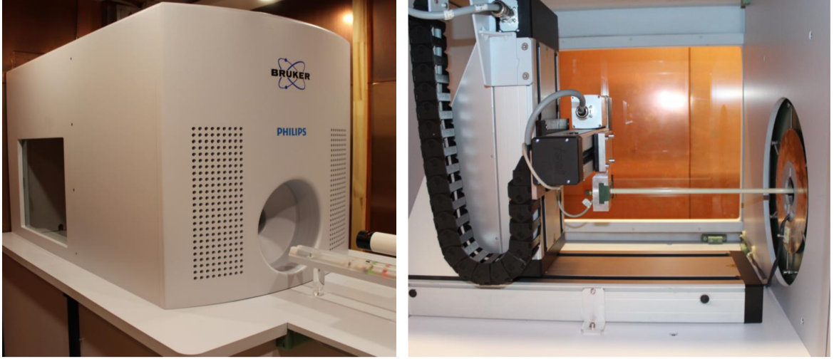
FIGURE 3.3: Left: MPI scanner frontend located inside the copper-shielded room. Right: Sample holder mounted to MPI calibration robot used for sample positioning and SF acquisitions.
