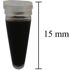
FIGURE 6.10: Photograph of one representative sample used for MPI and MRI measurements: Fast reaction tube filled with 160 \mu\text{L} Ferucarbotran diluted in water.
