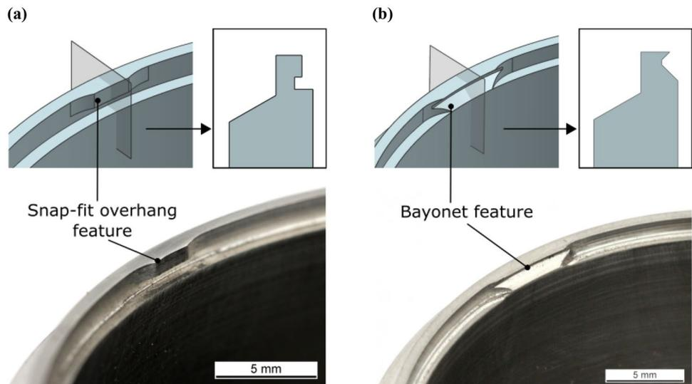
snap-fit pins appeared to deform plastically with every assembly iteration: After more than five assemblies, the interlocking became too weak to hold the specimen’s dead weight. Reliable handling and subsequent repeatable welding results can, therefore, can’t be guaranteed when the parts are disassembled multiple times.
