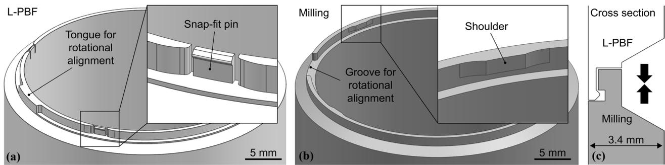
**Fig. 6** Snap-fit design with **a** L-PBF geometry with tongue and pin, **b** milling geometry with groove and shoulder, **c** schematic assembly design
