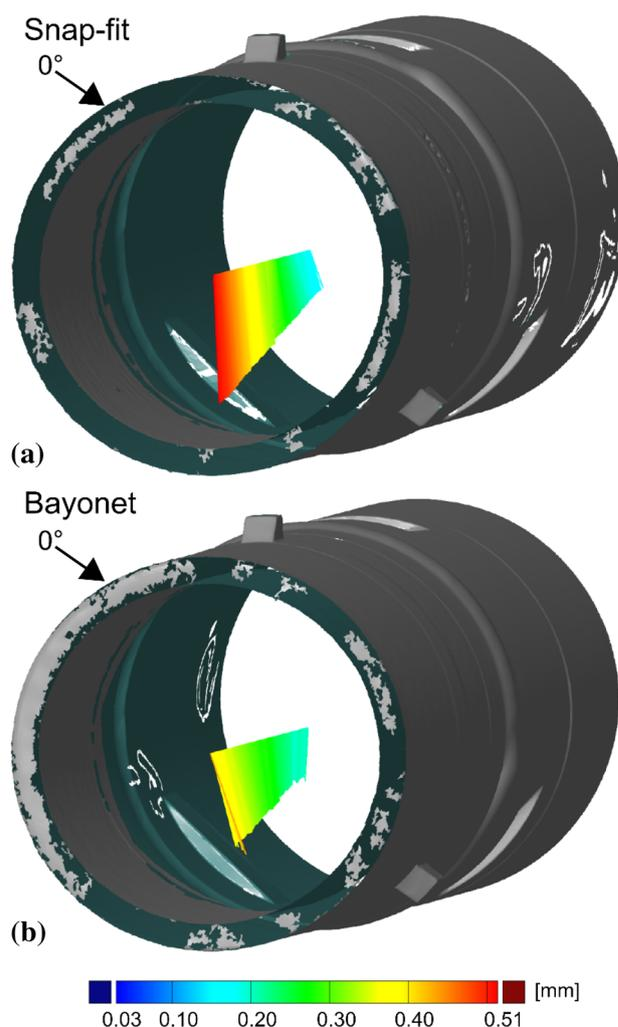
**Fig. 12** 3D scan results after welding of **a** snap-fit design and **b** bayonet design with measured center lines of the L-PBF cylinders in relation to the target center lines. A scaling factor of 30 for the shown deviations was used to improve visibility. 0° indicates the start position of the root weld
