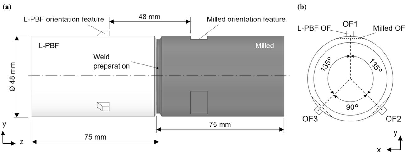
**Fig. 2** Specimen geometry **a** side view, **b** front view of an assembled pair of welding pipes with positions of orientation features (OF) used in all designs
