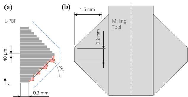
**Fig. 5** Geometric constraints for **a** L-PBF with a layer thickness of  $40\ \mu\text{m}$ , allowable overhang of  $45^\circ$ , min. wall thickness of 0.3 mm; **b** milling tool with a groove width of 0.2 mm, chamfer of  $45^\circ$ , max. depth of 1.5 mm; dimensions not to scale; expected L-PBF roughness in dashed red, ideal milling contour in dotted blue
