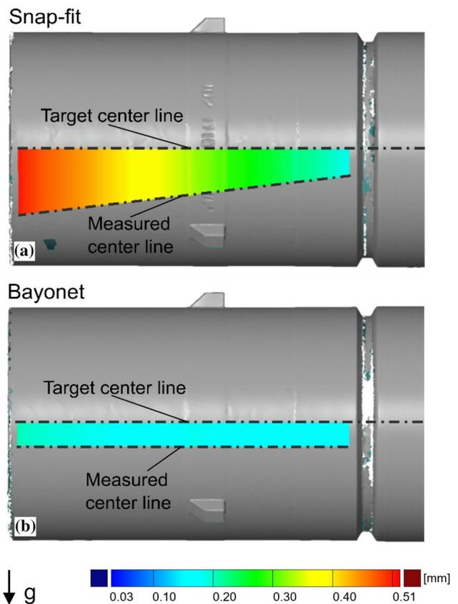
**Fig. 11** 3D scan results before welding of **a** snap-fit and **b** bayonet design with measured center lines of the L-PBF cylinders in relation to the target center lines. A scaling factor of 30 was applied to improve visibility
