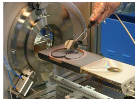
Figure A2.2 left: scheme of the growth chamber of a horizontal MOVPE reactor; right: the susceptor of an AIX-200 horizontal reactor is extracted from the growth chamber for wafer loading.
