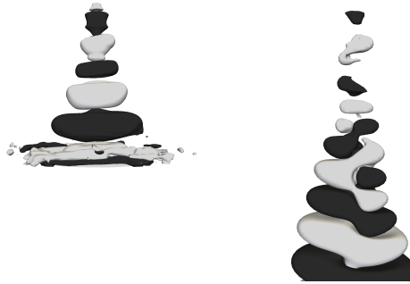
Figure 5.8: Pressure contours of the three-dimensional dynamic modes corresponding to the impinging tone (left, #1, Sr = 0.353 , p = \pm 0.05p_\infty ) and to screech (right, free jet, Sr = 0.375 , p = \pm 0.002p_\infty ).
