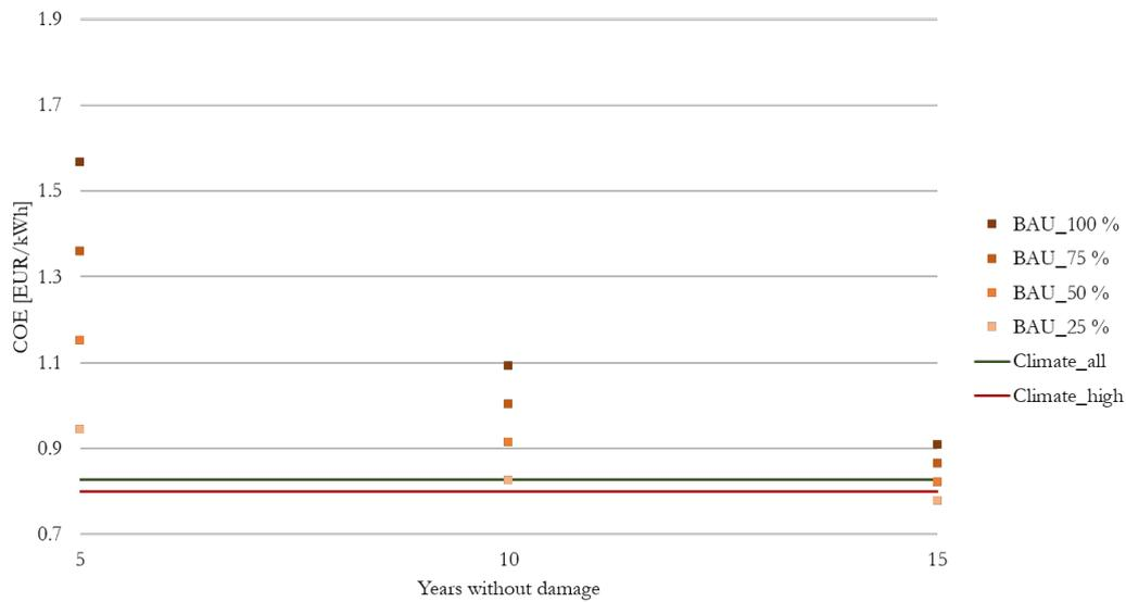
**Figure 4.30:** COEs for different evaluation scenarios (5, 10, and 15 years without damage as well as 25 %, 50 %, 75 %, and 100 % damage of each component) for the BAU system setup and reduced diesel fuel cost, Hon Son Cha island
