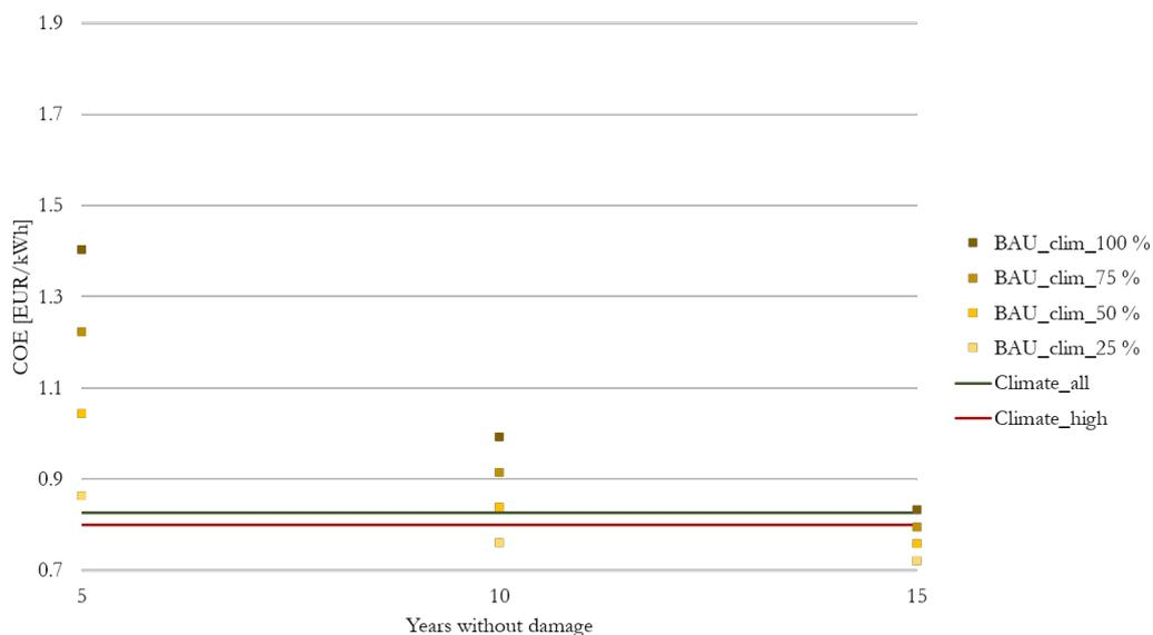
**Figure 4.31:** COEs for different evaluation scenarios (5, 10, and 15 years without damage as well as 25 %, 50 %, 75 %, and 100 % damage of each component) for the BAU system setup, climate demand and reduced diesel fuel cost, Hon Son Cha island
