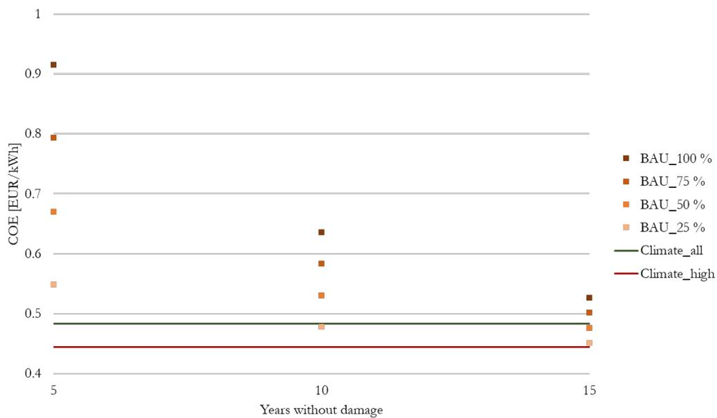
**Figure 4.26:** COEs for different evaluation scenarios (5, 10, and 15 years without damage as well as 25 %, 50 %, 75 %, and 100 % damage of each component) for the BAU system setup, Magyi Kyun island
