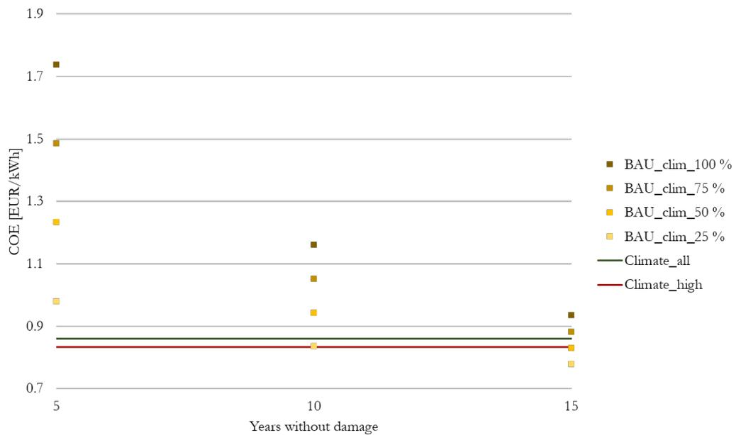
**Figure 4.25:** COEs for different evaluation scenarios (5, 10, and 15 years without damage as well as 25 %, 50 %, 75 %, and 100 % damage of each component) for the BAU system setup and climate demand, Hon Son Cha island
