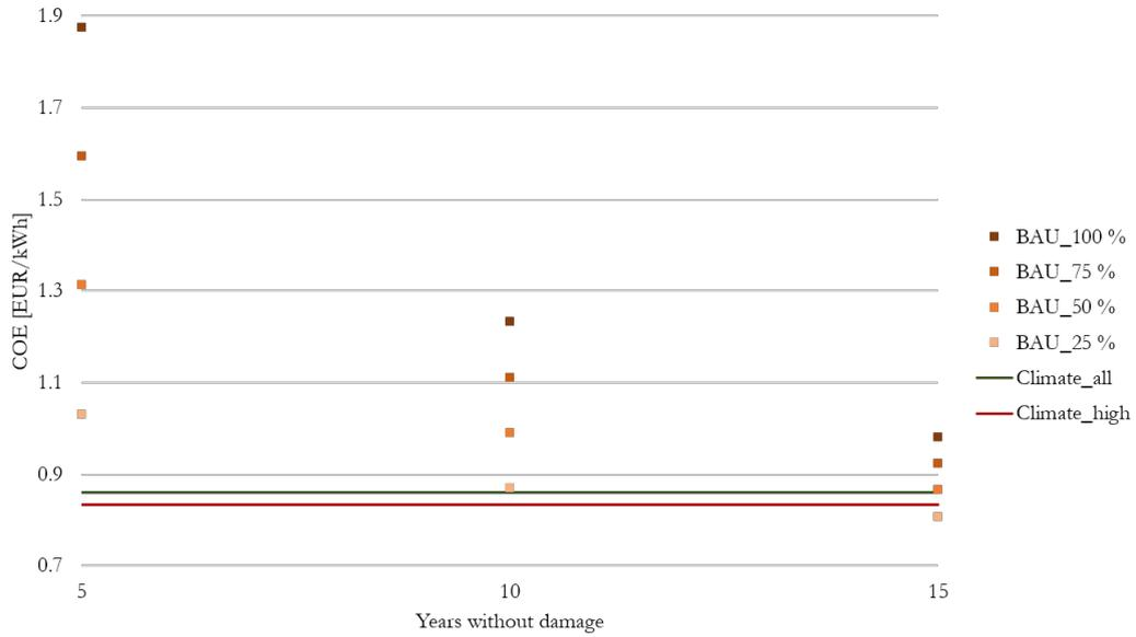
**Figure 4.24:** COEs for different evaluation scenarios (5, 10, and 15 years without damage as well as 25 %, 50 %, 75 %, and 100 % damage of each component) for the BAU system setup, Hon Son Cha island
