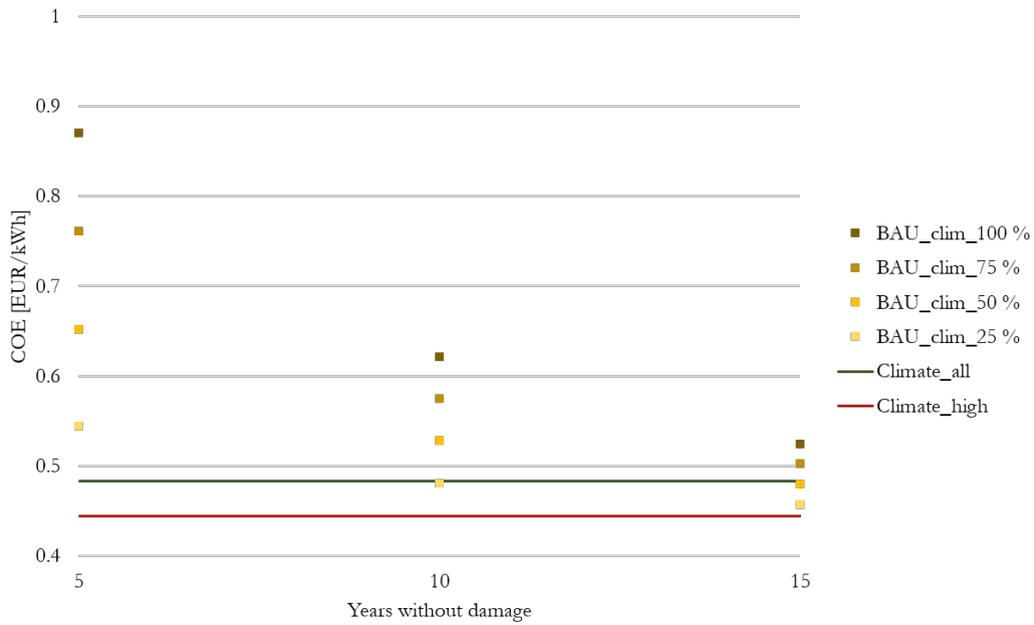
**Figure 4.27:** COEs for different evaluation scenarios (5, 10, and 15 years without damage as well as 25 %, 50 %, 75 %, and 100 % damage of each component) for the BAU system setup and climate demand, Magyi Kyun island
