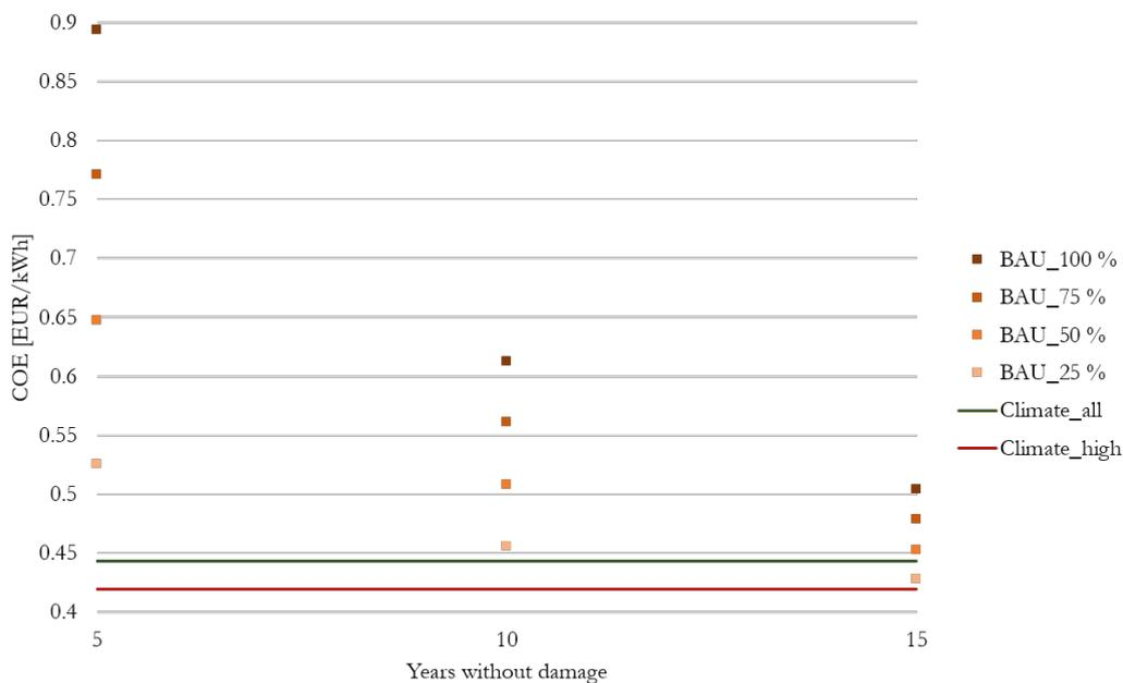
**Figure 4.28:** COEs for different evaluation scenarios (5, 10, and 15 years without damage as well as 25 %, 50 %, 75 %, and 100 % damage of each component) for the BAU system setup, Bulon Don island
