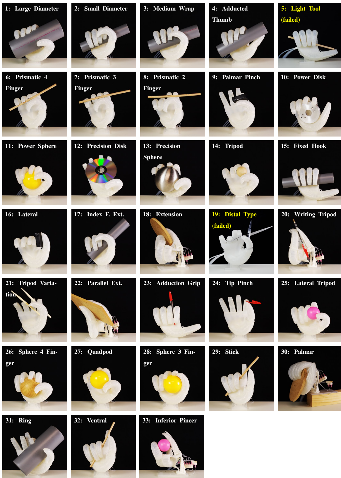
Fig. 8.9 Attempts to enact all grasps enacted from the Feix taxonomy [37], the hand failed to replicate grasps 5 (Light Tool) and 19 (Distal Type, Scissors). Images taken from Deimel and Brock [22] ©2016 Sage Publications
