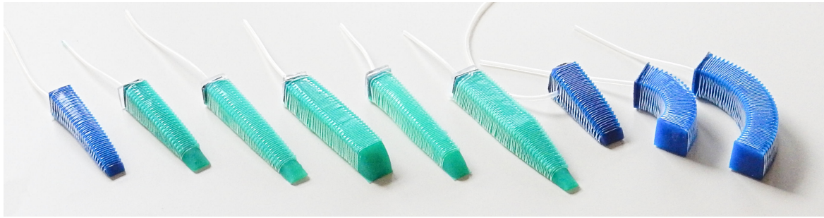
Fig. 3.6 The PneuFlex toolkit can be used to create actuators with many different but well defined mechanical behaviors.
