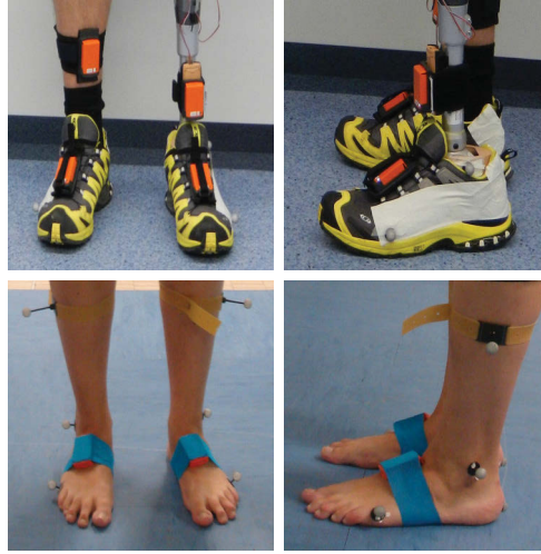
Figure 3.9: Experimental setup with IMUs and optical markers attached to shoes and bare feet. Note that the data of the IMUs that are attached to the shanks is not used in this study.
