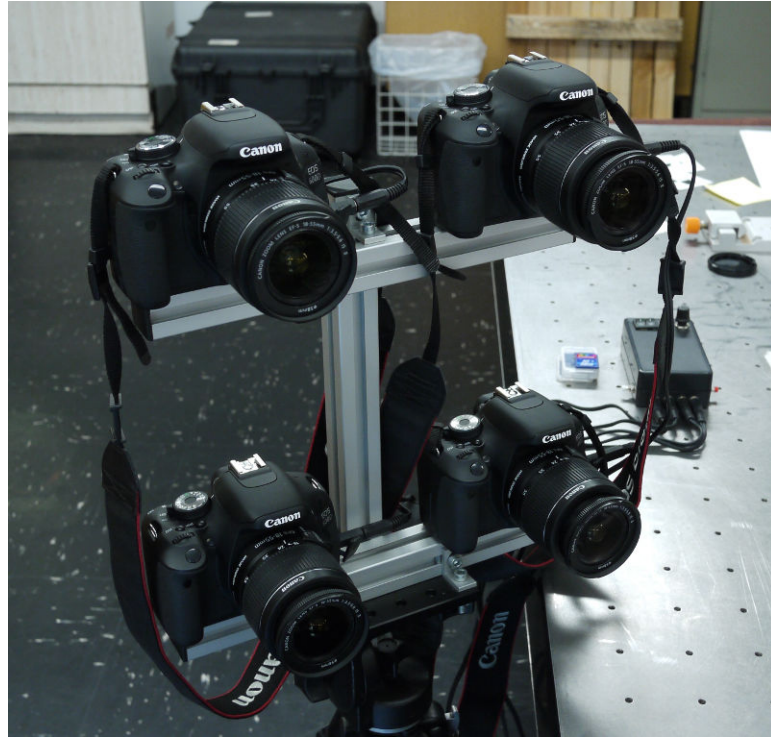
Figure 8.2: Quadrifocal camera setup to capture deformable objects.
