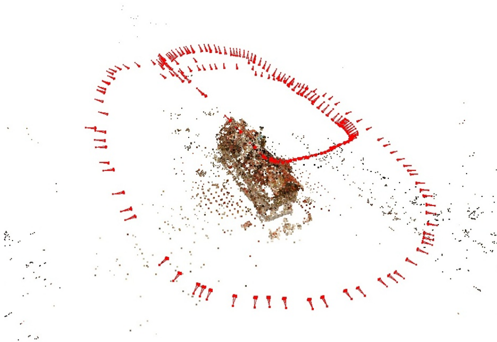
Figure 7.5: Reconstructed camera path with sparse point cloud.
