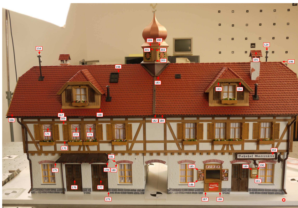
Figure 7.2: FTS with marked coordinates of GCP.
