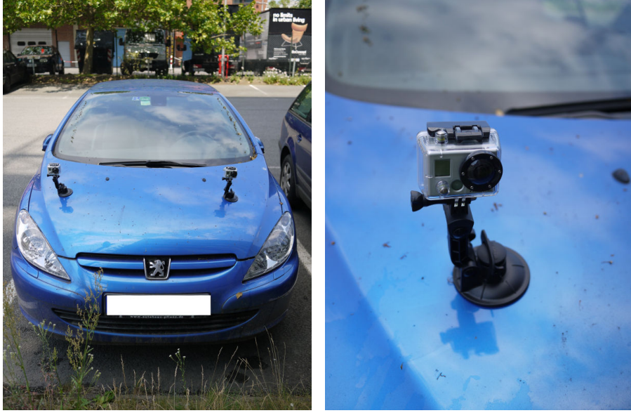
Figure 7.13: Acquisition setup with two GoPros on a car.
