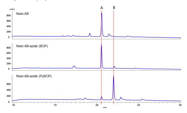
Supplementary Figure 1: HPLC analysis of reaction substrate nisin AB and the reaction mixtures using BOP and PyBOP. A: peak of substrate; B: peak of product. Conditions: RP 18 column  $4.6 \times 250$  mm, solvent A,  $H_2O$  with 0.1% TFA; solvent B, acetonitrile with 0.1% TFA; flow rate 1 mL/min for a 45 min run. A gradient (0-5 min 20% solvent B, 5-30 min linear to 60% solvent B; 30-31 min linear to 100% solvent B and within 45 min back to 20% solvent B) was used.
