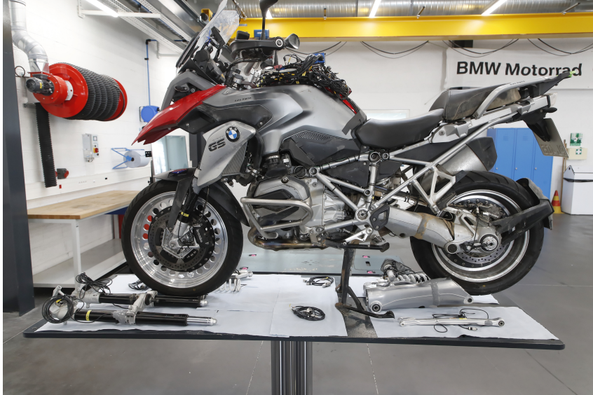
Figure 1.3 – Exemplary measurement motorcycle with wheel load transducers ©BMW AG.
