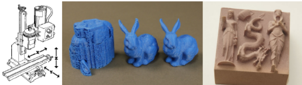
Figure 6.1: Left: 3-axis milling machine with limited degrees of freedom introduces limitations for additive and subtractive manufacturing. Middle: Most 3D printing techniques need support material to strut overhanging structures. Right: The geometric complexity of 3-axis CNC milling is limited.
