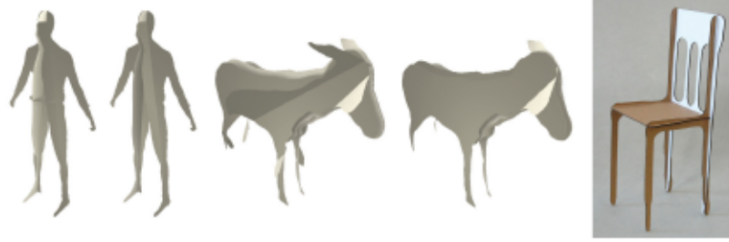
Figure 7.6: Left, middle: Given a set of planes generated by McCrae et al. [2011] we apply our insertion strategy in an optimal (left) and not optimal (right) construction case. Right: Cardboard model [McCrae et al. 2011]
