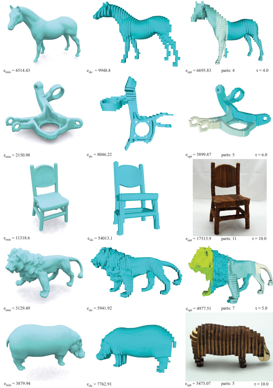
Figure 5.17: We show the input 3D shapes (left), a result that is sliced in its best direction (middle) and the handcrafted or 3D printed results or rendered images (right). We also show the best approximation error, the error that would result from one directional slicing and the error after optimization. Additionally parameter settings and the number of resulting subparts are annotated.
