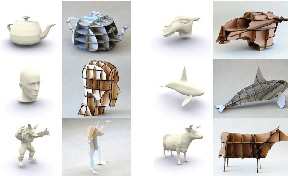
Figure 7.17: Resulting cardboard sculptures created from a completely automatic two-step process. The first step finds to best planar section based on the plane quality evaluation presented in Section 7.3 . In the second step we additional sample axis-aligned planes. The Armadillo is created only of planar sections from the plane quality based sampling.
