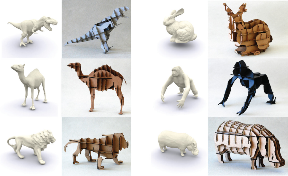
Figure 7.16: We show the input meshes and the handcrafted cardboard models using axis-aligned grid sampling to find a set of planes. The process for all models is automatic except for the gorilla where we added an additional plane manually.
