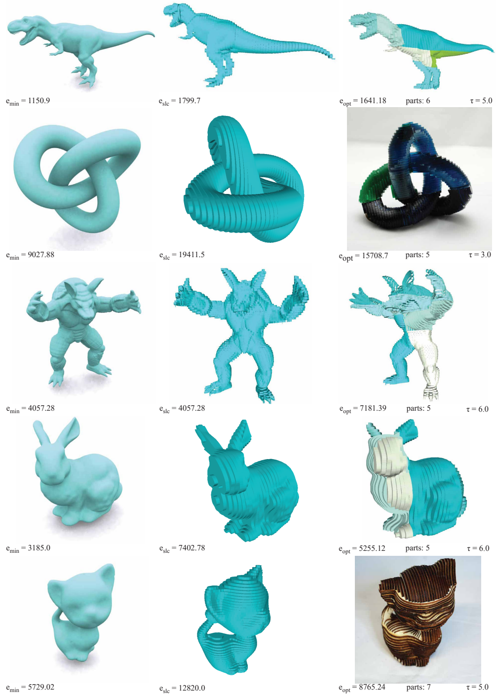
Figure 5.18: We show the input 3D shapes (left), a result that is sliced in its best direction (middle) and the handcrafted or 3D printed results or rendered images (right). We also show the best approximation error, the error that would result from one directional slicing and the error after optimization. Additionally parameter settings and the number of resulting subparts are annotated.
