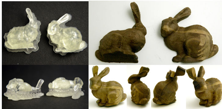
Figure 6.2: Left: Two parts of the input shape are printed separately using stereolithography. The needed support material for an FDM print is decreased compared to an a single part along an up-right direction. Right: A 3D shape out of wood fabricated in two pieces using a CNC milling machine. The fabrication error is minimized by the choice of the partitioning plane.
