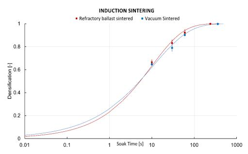
**Figure 8.** Johnson–Mehl–Avrami–Kolmogorov (JMAK) model curves of the 316L FFF parts sintered within the refractory ballast (red), and in a vacuum (blue).
