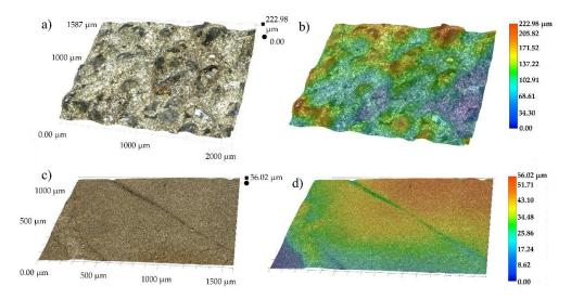
**Figure 18.** 3D surface topography measurements at mag.  $200 \times$  for specimens sintered within (**a**) the refractory ballast with (**b**) color-coded, and (**c**) vacuum-sintered with (**d**) color-coded.
