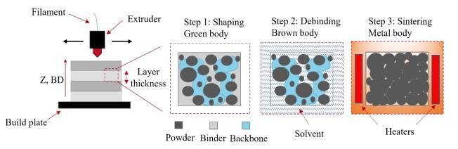
Figure 1. Illustration of the FFF processing steps to produce dense metal or ceramic parts.
