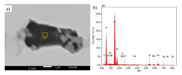
**Figure 16.** EDX measurement within a void in the sample sintered in (**a**) refractory ballast for 240 s and (**b**) the chemical composition of the refractory of the refractory ballast sintered.
