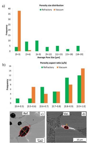
**Figure 9.** (a) Mean porosity size as a function of frequency and (b) porosity aspect ratio for the refractory-sintered (green) and vacuum-sintered (orange) specimens. Subfigures (c,d) show the shape of the porosities for the refractory ballast and vacuum sintered, respectively, with the measured semi-minor axis, a, and semi-major axis, b, indicated within the micrographs.
