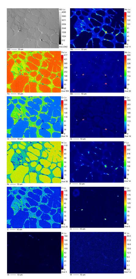
**Figure 14.** WDX measurement for the vacuum-sintered for 360 s, mapping Fe, Cr, Ni, Mo, Mn, Si, P, C, O, Al, and W.
