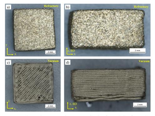
**Figure 17.** Indirect induction sintered specimens within the refractory ballast for a soak time of 240 s in the (a) XY and (b) ZX planes, and vacuum sintered for a soak time of 360 s in the (c) XY and (d) XZ planes.
