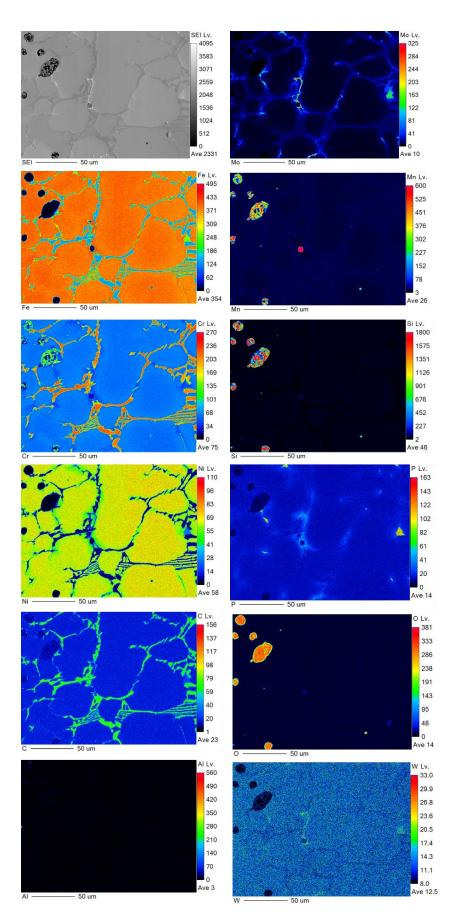
**Figure 13.** WDX measurement for the refractory ballast sintered for 240 s, mapping Fe, Cr, Ni, Mo, Mn, Si, P, C, O, Al, and W.
