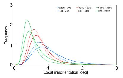
**Figure 12.** Local misorientation distributions of the refractory ballast (solid lines) and vacuumsintered (dashed lines) samples.
