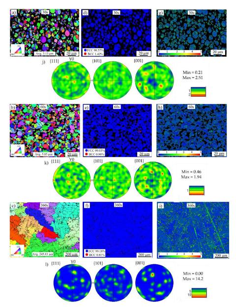
**Figure 11.** EBSD maps of the vacuum sintered specimens after (**a**) 30 s, (**b**) 60 s, and (**c**) 360 s, phase maps of the specimens after (**d**) 30 s, (**e**) 60 s, (**f**) 360 s, local misorientation maps after (**g**) 30 s, (**h**) 60 s, (**i**) 360 s and Euler pole figures after (**j**) 30 s, (**k**) 60 s, and (**l**) 360 s.
