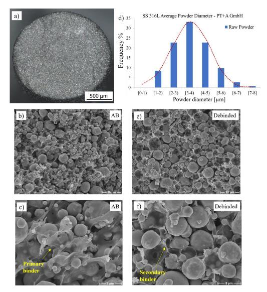
**Figure 3.** (a) Raw filament cross-section at mag.  $50 \times$ , (b) micrograph of feedstock with stainless steel 316L powder embedded by polymeric binder at mag.  $1000 \times$  and (c) mag.  $3000 \times$ , (d) particle size distribution of measured powder in the debinded state, (e) micrograph of the debinded geometry at mag.  $1000 \times$  and (f) mag.  $3000 \times$ .
