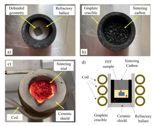
**Figure 5.** Indirect induction sintering setup with (**a**) the debinded geometry partially buried in the refractory ballast, (**b**) graphite crucible with a top layer of carbon pellets, (**c**) treatment in operation, and (**d**) illustration of the test.
