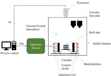
Figure 2. Illustration of the hybrid FFF and indirect induction sintering enabling in situ processing.
