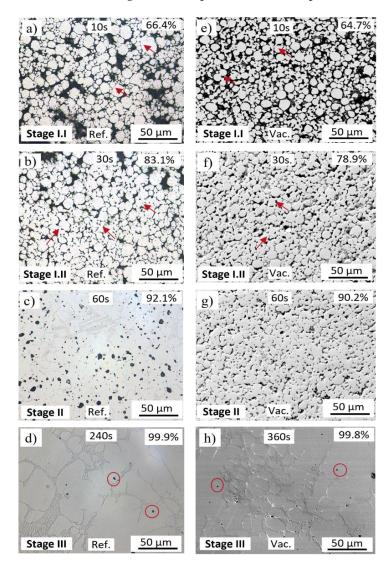
**Figure 7.** Micrographs of the indirect induction sintered FFF 316L stainless steel in the refractory ballast after (**a**) 10 s, (**b**) 30 s, (**c**) 60 s, and (**d**) 240 s, and sintered in the vacuum tube after (**e**) 10 s, (**f**) 30 s, (**g**) 60 s, and (**h**) 360 s.
