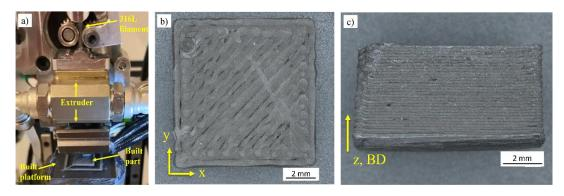
**Figure 4.** (a) Custom in-house FFF machine shaping a geometry, (b) XY plane of AB green parts and (c) Z-BD plane.
