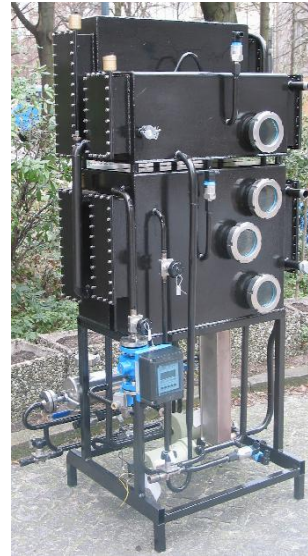
Figure 1: Prototype of a 10 kW absorption chiller and technical data
