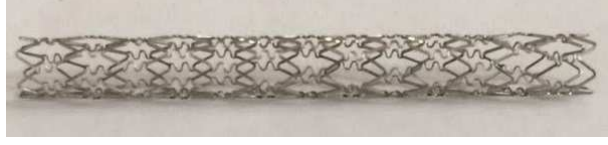
Figure 1: Example of an elastic stent (Cypher stent by Cordis Corporation)
